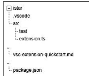
Figure 2 - File structure provided for a extension called istar of type extension (Typescript) .
