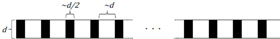
**Figure 1.3:** Painting pattern of the duct to assist its detection in the images.
