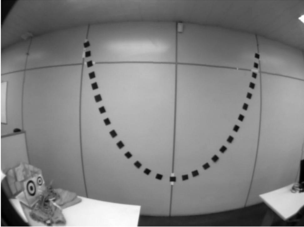
**Figure 5.1:** An example of a frame from the laboratory videos. The catenary was represented with a sequence of black squares to be detected by the same algorithm that detects ducts in the real application. (Source: The author)
