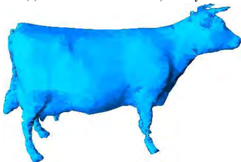
7(a): base mesh : threshold 3.0, 2258 bytes
