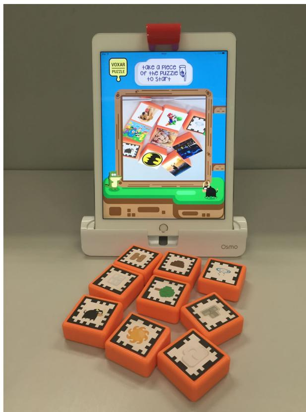
Figure 1: AR jigsaw running on Voxar Puzzle. Note that the iPad is on the Osmo's tablet support and the mirror is the red object covering the frontal camera.
