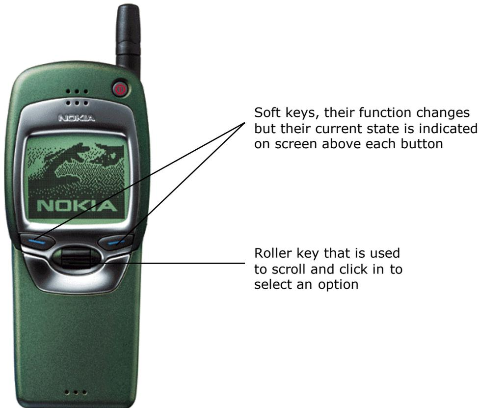
The current function is displayed on screen. If the soft keys are pressed, menus offering further options (such as “Exit” or “Go to main menu,” etc.) are displayed. To a large degree, these soft keys provide macro navigational assistance, whereas the roller key provides the micro navigational capacity needed to move toward a specific WAP site. The key pad is behind the cover, which can be slipped down when needed.
