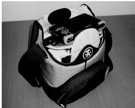
Figure 11. The most recent version of the field laboratory weighing only 2 kg and measuring just 18x14x25 cm—containing video and audio receivers, Picture-in-Picture unit, hard disk recorder, and battery.
