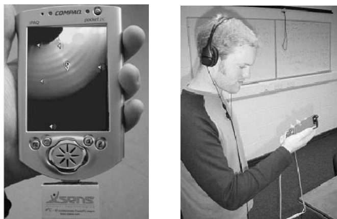
Figure 3. Left- Pocket PC, Accelerometer and experiment I running on the system (target sound sources displayed, for illustrative purposes). Right- A user interacting with the system.
