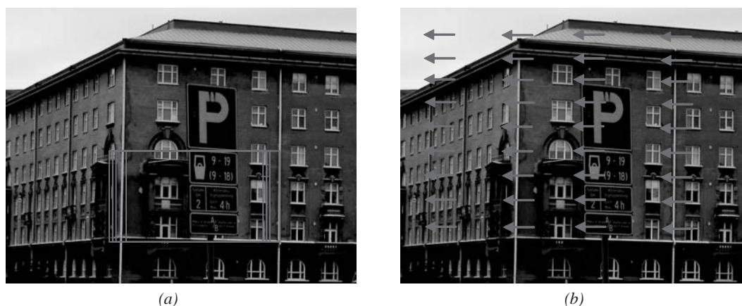
Figure 1. Motion simulation. A base image with sliding window locations on the left (a) and a frame with ground truth motion (b) on the right.
