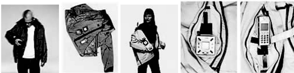
Figure 6. Incorporating consumer electronics into clothing—the Philips-Levi Strauss jacket 4
