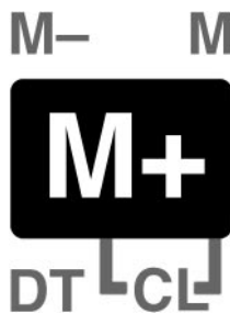
FIGURE 1. Schematic of the \boxed{\text{M+}} key. The key is black with M + in white. The labels M- and CL are in yellow; the M (top right) in red; and the DT and lines underneath are in blue. The SD mode (“standard deviation”) uses blue labels, and the shifted functions are yellow: the colour coding of the CL function is meant to indicate that in SD mode, a shifted \boxed{\text{M+}} press obtains the function CL , not M- .
