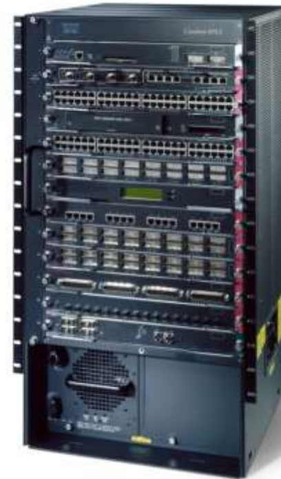
Central Core Switch
