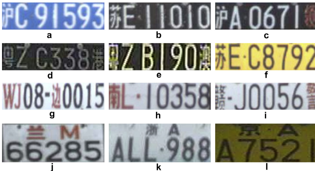
Fig. 1. Main vehicle license plate types in Mainland China: (a) blue; (b) black (foreign institution); (c) black (consulate); (d) black (Hong Kong); (e) black (Macao); (f) yellow (installed in the front of vehicles); (g) white (armed police); (h) white (military); (i) white (police); (j) white (military); (k) white (civilian) and (l) yellow (installed at the back of vehicles).
