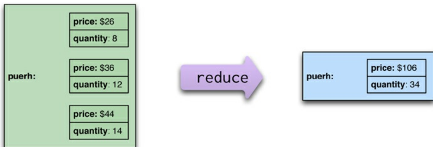
Figure 7.2. A reduce function takes several key-value pairs with the same key and aggregates them into one.
