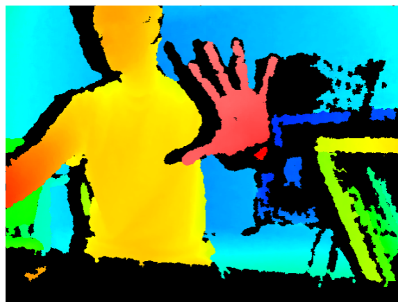
Figure 17: A depth image from the Microsoft Kinect.
