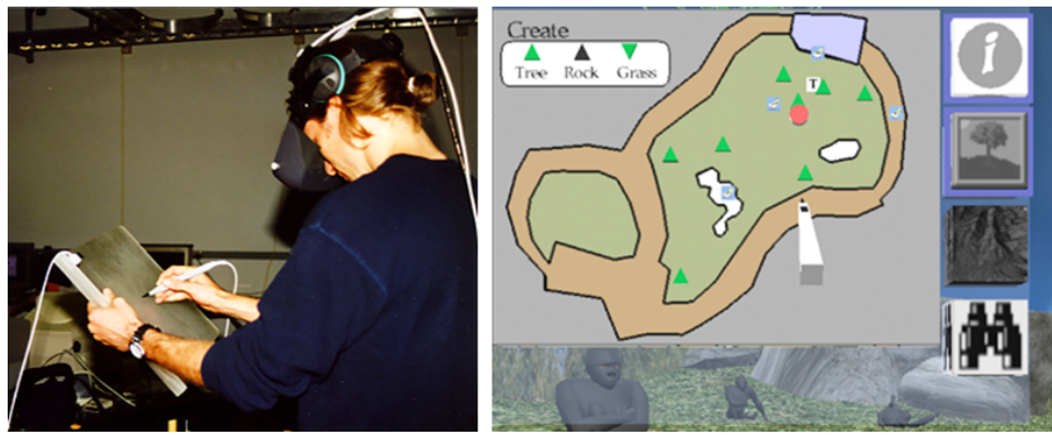
Figure 10: The Pen and Tablet Metaphor. The image on the left shows the user holding the pen and tablet and the image on the right shows what the user's sees in the virtual world.
