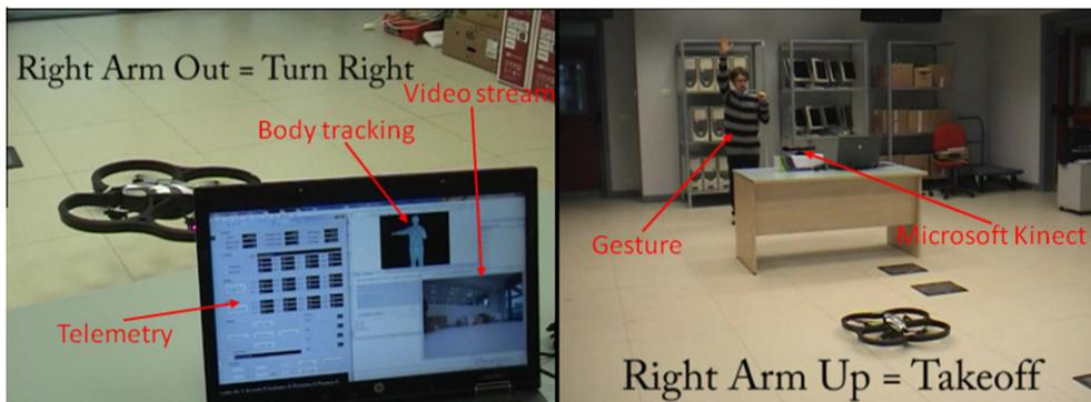
Fig. 4. Screen of the control station (left) and flying platform (right).
