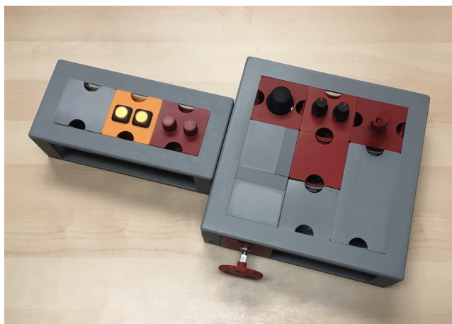
Figure 11: Two Probatio bases assembled with blocks. Red blocks provide continuous inputs, the orange one hosts two discrete buttons. Grey blocks are dummy blocks to keep the structure in place.
