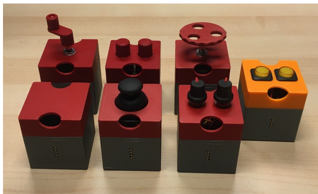
Figure 10: 3D printed probatio -blocks. From left to right upper row: crank, dual pistons, dial, dual buttons (in orange). Bottom row: piezo tap, joystick, dual potentiometers
