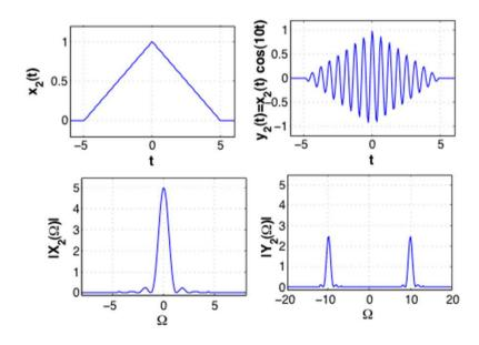
Why Modulation? Modulation changes frequency content of a message from its baseband frequencies to higher frequencies making its transmission over the airwaves possible
