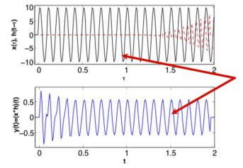
input sinusoid ss output sinusoid of same frequency
