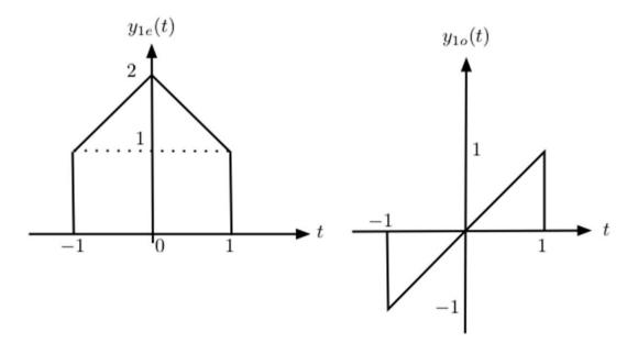
Signal y(t) neither even nor odd, cannot be made even or odd by shifting Even and odd components of period  $y_1(t)$ ,  $-1 \le t \le 1$ :
