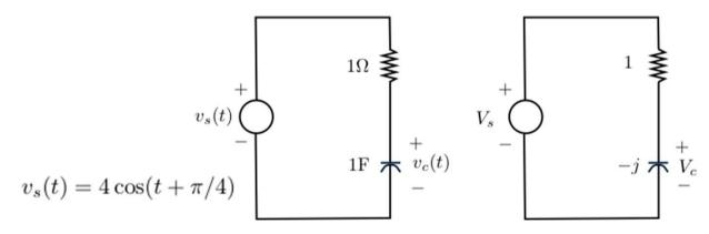
Phasor Approach:  $V_s = 4 \angle \pi/4$  phasor for  $v_s(t)$ ,  $V_c$  phasor for  $v_c(t)$
