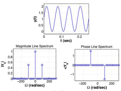
Line spectrum of Fourier series of  $y(t) = 1 + \sin(100t)$ . Notice the even and the odd symmetries of the magnitude and phase spectra. The phase is  $-\pi/2$  at  $\Omega = 100$  (rad/sec).
