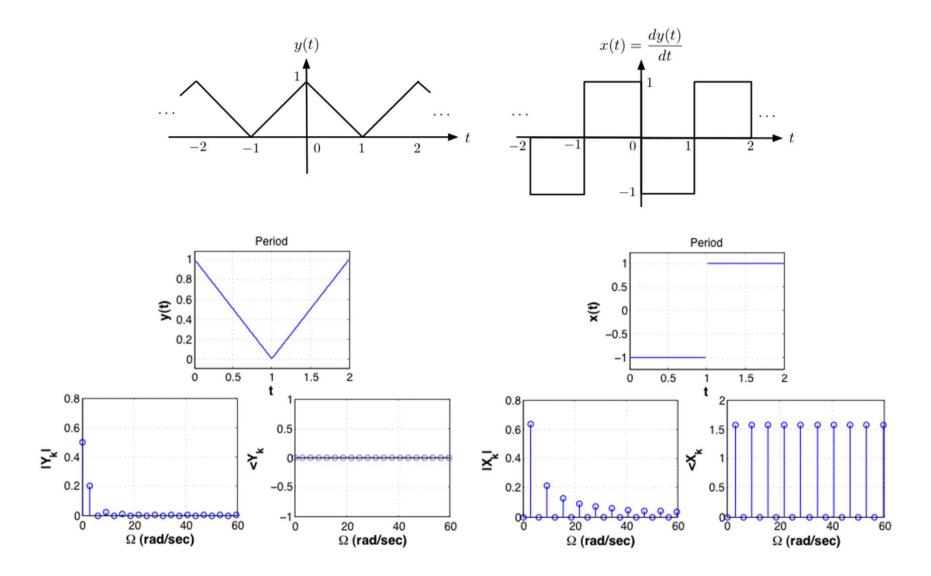
Example Effect of integration: compare the magnitude line spectra of a saw-tooth signal x(t), of period  $T_0 = 2$ , and its integral
