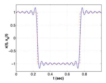
Approximate Fourier series  $x_N(t)$  of the pulse train x(t) (discontinuous) using the dc component and 20 harmonics. The approximate  $x_N(t)$  displays the Gibb's phenomenon around the discontinuities.
