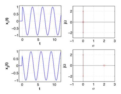
Location of the poles and zeros of  $\cos(2t+\theta)u(t)$  for  $\theta=0$  (top figure) and for  $\theta=\pi/4$ . Note that the zero is moved to the right to 2 (the value of the frequency) because the zero of the Laplace transform is  $s=\Omega_0\tan(\theta)=2\tan(\pi/4)=2$ .
