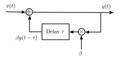
Input/output equation  $y(t) = x(t) + \beta y(t - \tau)$  if  $x(t) = \delta(t)$ , the output y(t) = h(t) or
