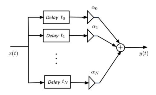
$$y(t) = \alpha_0 x(t - t_0) + \alpha_1 x(t - t_1) + \dots + \alpha_N x(t - t_N)$$
