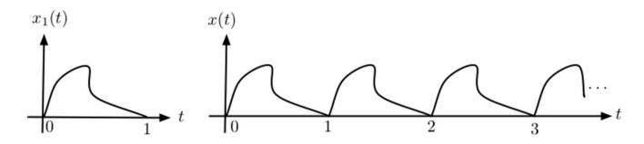
Example Find Laplace transform of causal full-wave rectified signal First period
