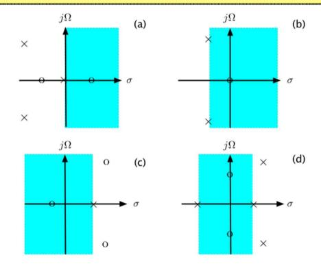
ROC for (a) causal signal with poles with  $\sigma_{max} = 0$ ; (b) causal signal with poles with  $\sigma_{max} < 0$ ; (c) anti-causal signal with poles with  $\sigma_{min} > 0$ ; (d) two-sided or noncausal signal where ROC is bounded by poles (poles on left-hand plane give causal component and poles on the right-hand s-plane give the anti-causal component of the signal)
