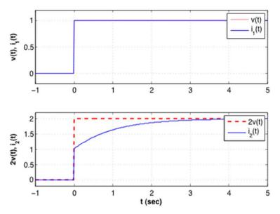
Non-linear behavior of RL circuit:  $I_0 = 1$ , B = 1, v(t) = u(t),  $i_1(t) = u(t)$  (top) and  $I_0 = 1$ , B = 2, v(t) = 2u(t),  $i_2(t) = (2 - e^{-t})u(t)$  (bottom),  $i_2(t) \neq 2i_i(t)$ .
