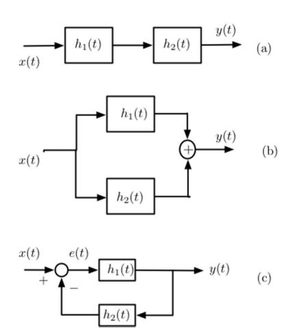
Block diagrams for connecting two LTI systems with impulse responses  $h_1(t)$  and  $h_2(t)$  in (a) cascade, (b) parallel, and (c) negative feedback.
