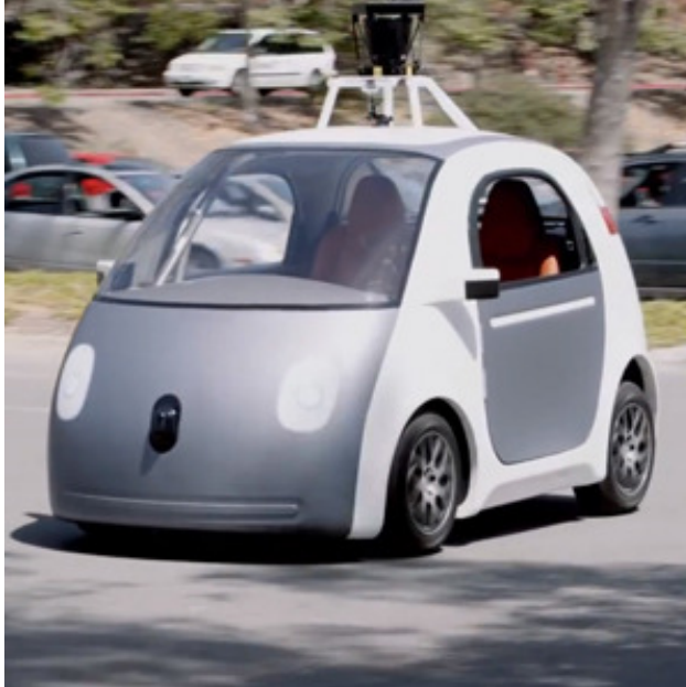
Passenger vehicle: A prototype car, demonstrated by Google in May of this year, that lacks a steering wheel or pedals.
