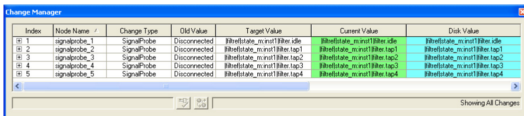
Figure 12-5. Change Manager Window with SignalProbe Pins
