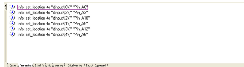
Figure 1–13. Equivalent Tcl Commands Displayed in the Messages Window
