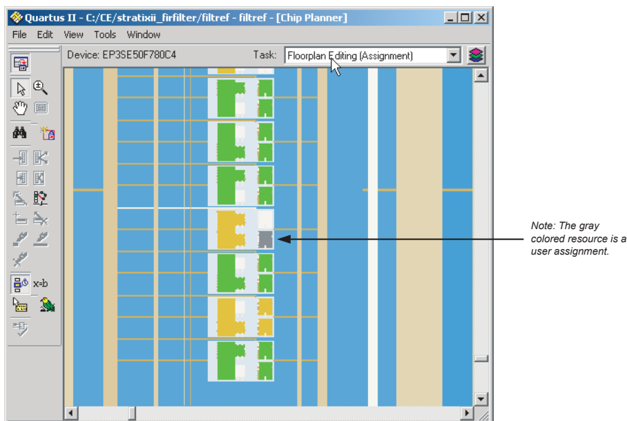
Figure 10–23. Viewing Assignments in Chip Planner
