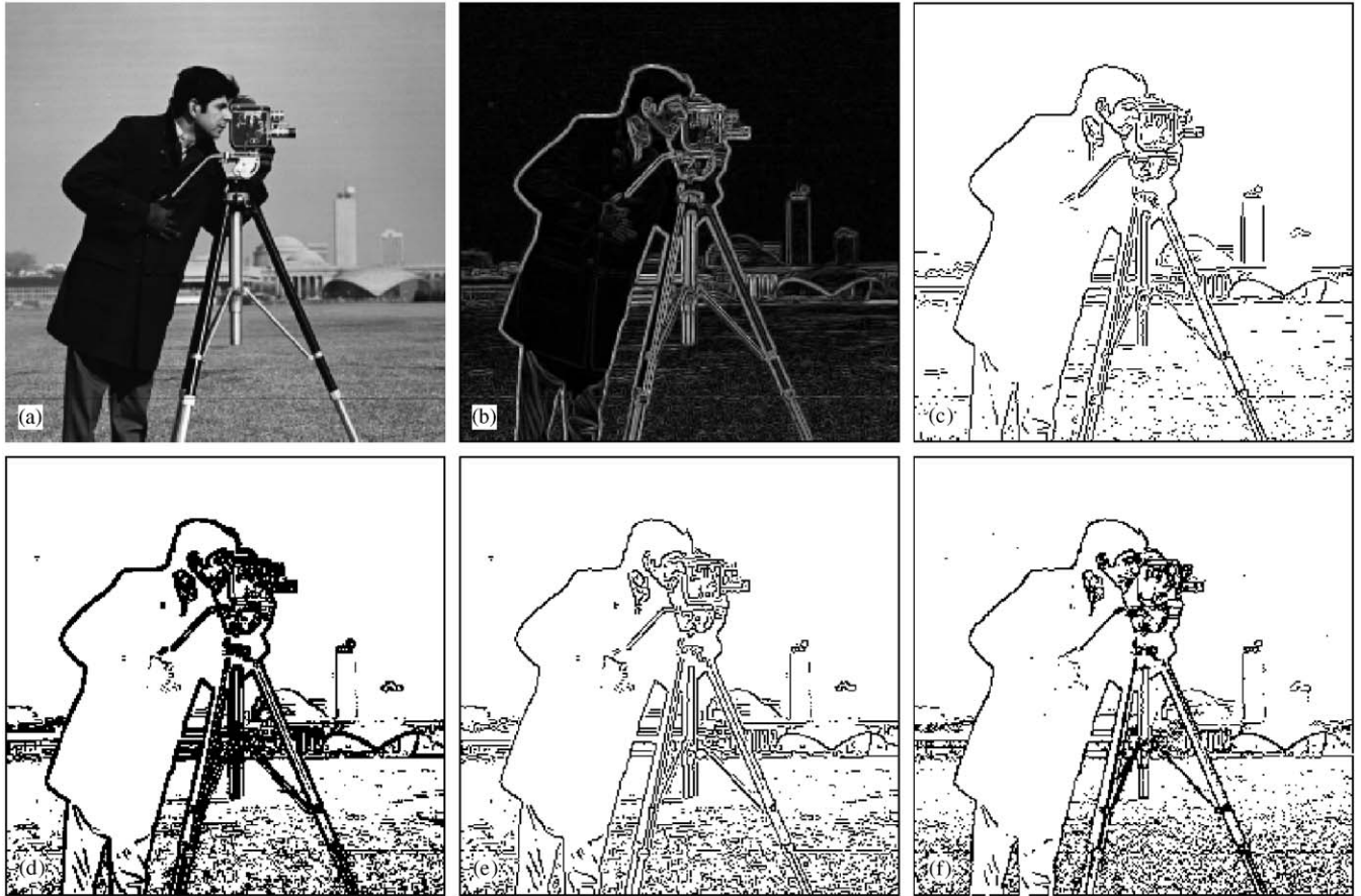
Fig. 9. Comparisons with different methods for “cameraman” image: (a) the original “cameraman” image; (b) the edge map by using the proposed method with w_1 = 90 , w_2 = 40 ; (c) the result of the proposed method with T = 50 ; (d) the result of Sobel method with T = 120 ; (e) the result of Canny method with T = 120 ; (f) the result of CFED with l_o = 8 , h_i = 50 , and w = 240 .
