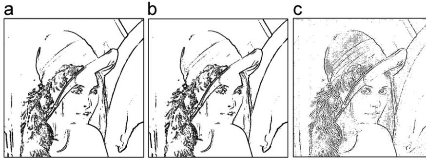
Fig. 4. Edge maps of the Lena image: (a) the present detector with mask = 3,  $C = 1$  (b) the Sobel detector, and (c) the LOG detector.
