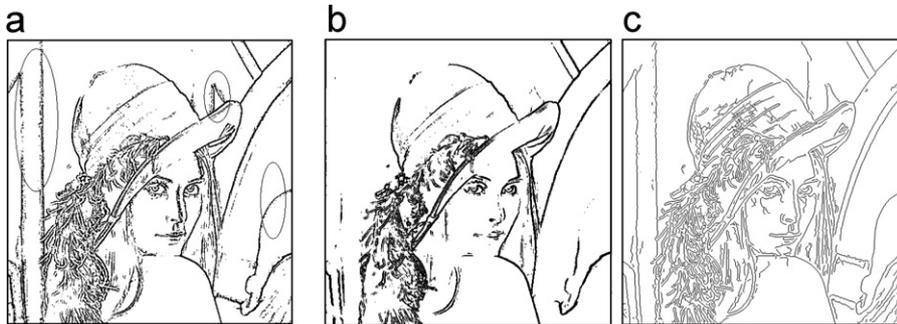
Fig. 5. Edge maps of the Lena image: (a) the present detector with mask = 3,  $C = \text{sig}(g(i, j))$ , (b) the Sobel detector, and (c) the Canny detector.
