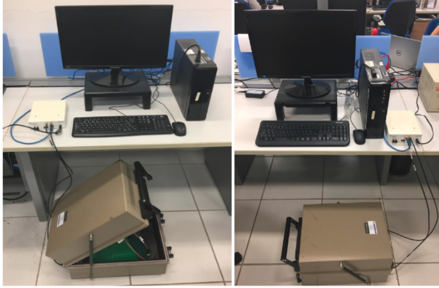
Figure 3: USRP-based Testbed to instance the proposed architecture.
