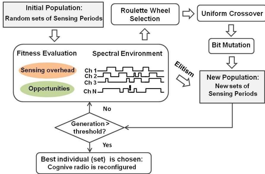
Figure 7. Execution Flow of the Scheme Based on GA.
