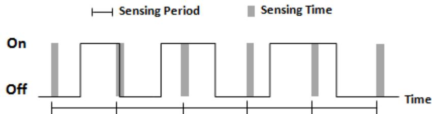
Figure 1. ON-OFF Model and Sensing Time and Sensing Period Concepts
