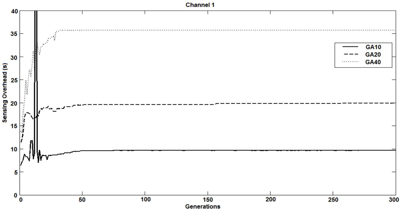
Figure 11. Sensing Overhead in the Channel 1
