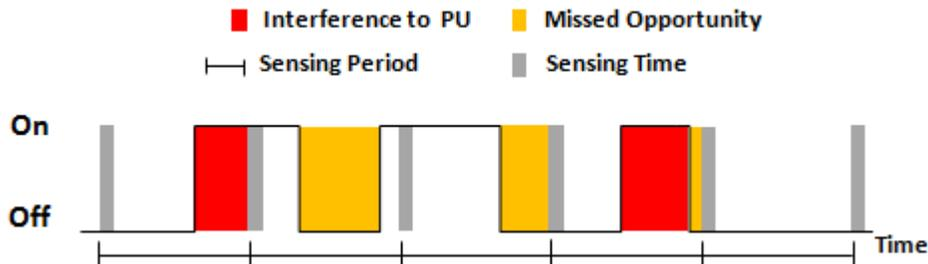
Figure 3. Larger sensing period may result in lower performance and thus interference to PU
