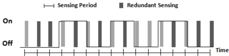
Figure 2. Redundant sensing leads to too much overhead
