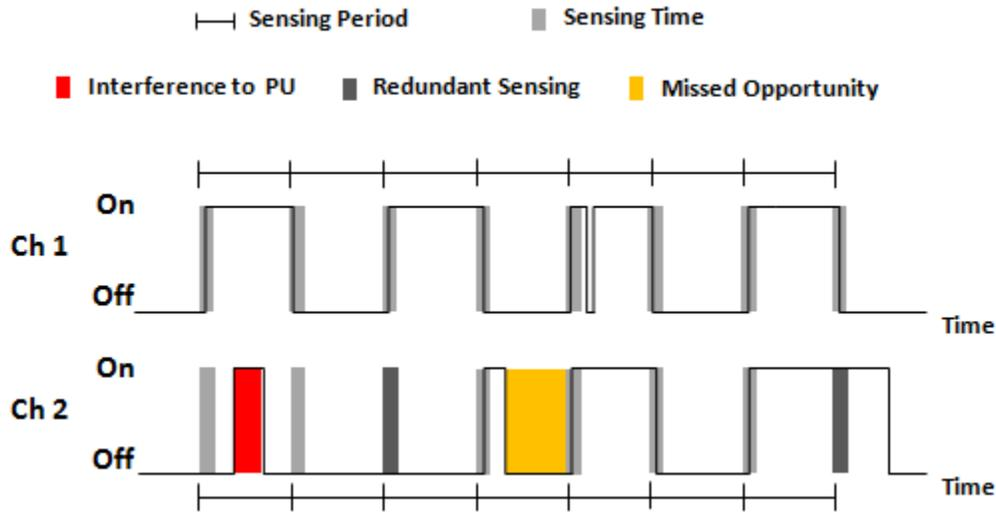
Figure 4. A single sensing period for all channels: effective for channel 1 but not effective for channel 2
