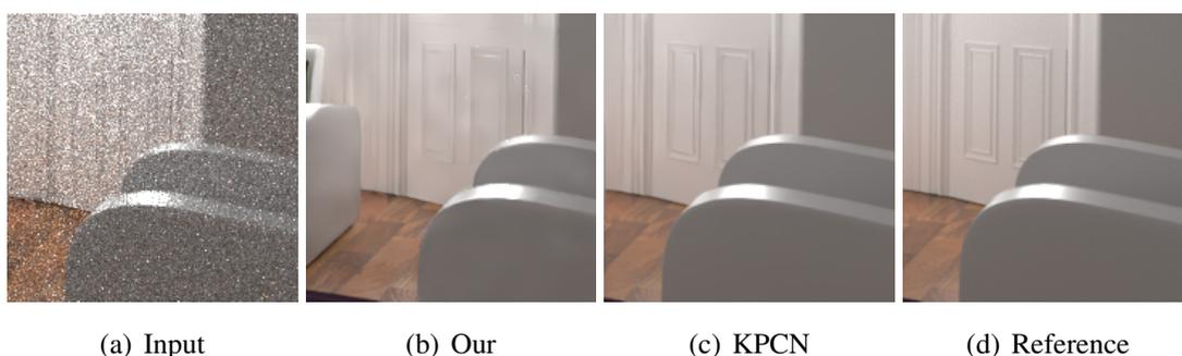
**Figure 6.6:** Comparison of our denoiser performance on the *White Room* scene. As we can see, in this case, our denoiser produces some undesirable patterns in the image and removes fine details of the door. On the other hand, the KPCN filters do not suffer from these stranger patterns at all but we see that the KPCN also removes some details from the image.
