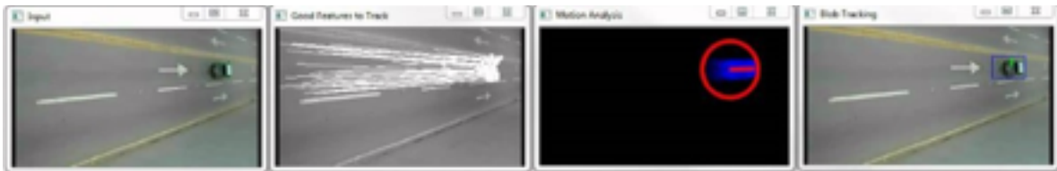
Figure 2: Example of a background subtraction algorithm in an automatic traffic analyser. Image obtained from (Ferreira 2016)
