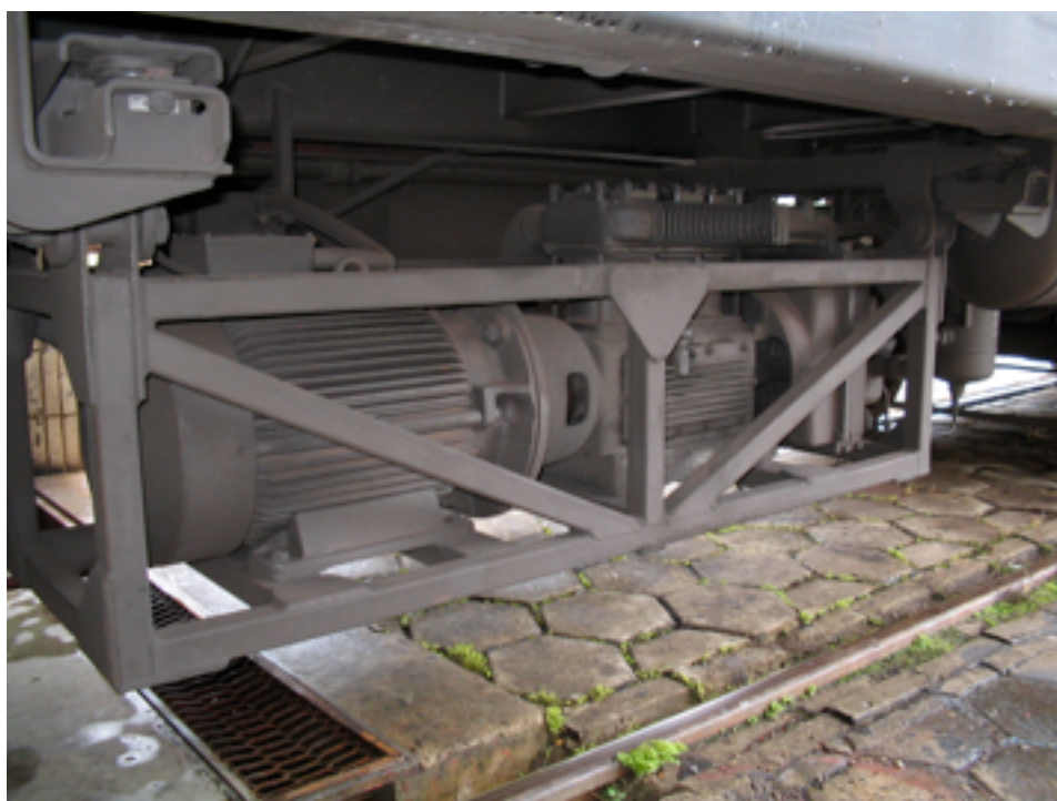
Figura 3-19. Compressor Principal (CBTU/METROREC, 2009).
