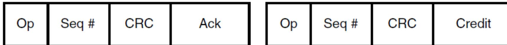
EFCP Control PDUs: Synch, Ack, Flow Control
