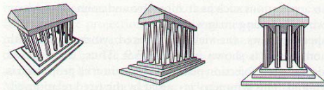
Figure 5.10 Classical perspective views: The (a) three-, (b) two-, and (c) one-point perspectives.
