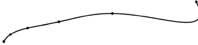
Figure 6.3: Lagrange interpolation: while the data points suggest a convex interpolant, the Lagrange interpolant exhibits extraneous wiggles.
