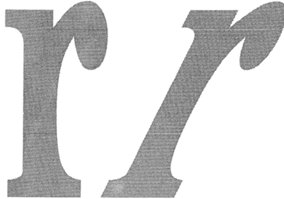
Figure 2.4: A shear: this affine map is used in font design in order to generate slanted fonts. Left: original letter; right: slanted letter.
