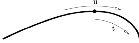
Figure 12.11: G^r continuity: a segment of a C^r may be reparametrized. The resulting curve is not C^r any more, but still G^r .
