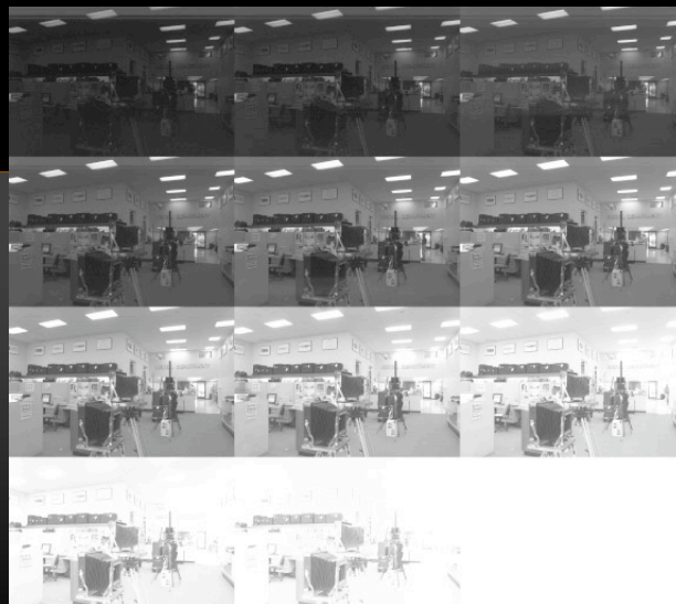
Eleven grayscale photographs of an indoor scene acquired with a Kodak DCS460 digital camera, with shutter speeds progressing in 1-stop increments from 1/30 of a second to 30 seconds.
