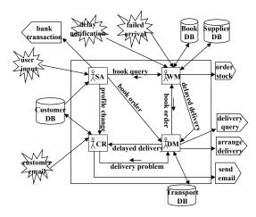
The final aspect of the architectural design is to specify fully the *interaction* between agents. Interaction diagrams are used as an initial tool for doing this, while fully specified interaction protocols are the final design artifact.
