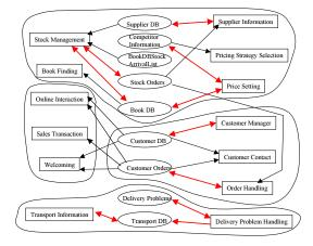
The diagram can be checked to ensure that all data is produced somewhere, unless it has been determined that it is provided externally on system start-up and is static. Also, the existence of data that is produced but not used usually indicates an omission elsewhere in the design.
