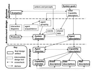
Figure 1. Phases, artifacts and relationships in the design process
