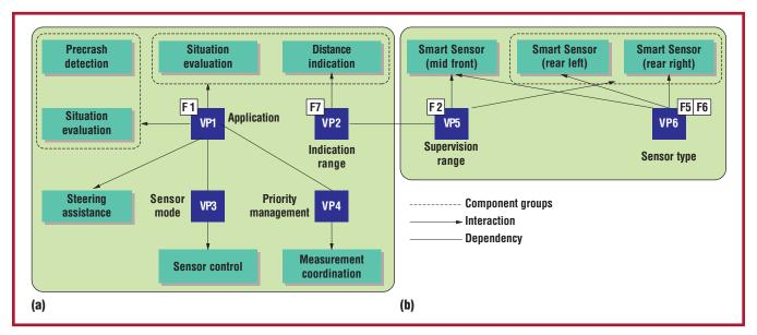
Figure 3. Variability in the (a) logical architecture and the (b) physical architecture. The variation points satisfy the variability among the requirements in Figure 2. "F" indicates a feature and "VP" a variation point.
