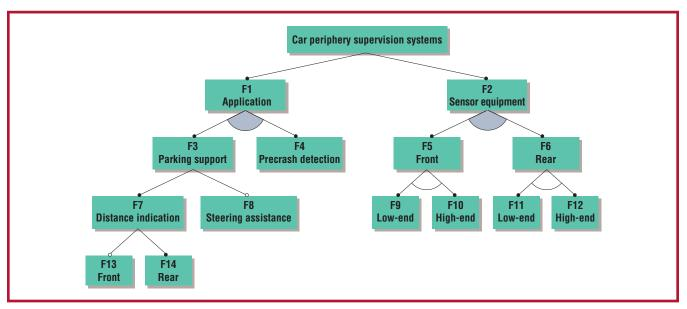
Figure 2. A feature model for a product line that provides car periphery supervision, which uses sensors to detect objects in the vehicle's environment. "F" indicates a feature. Filled arches indicate or-features and empty arches indicate alternative features; filled circles indicate mandatory features and empty circles indicate optional features.<sup>10</sup>
