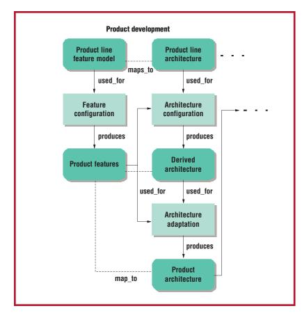
Figure 4. Interaction between the feature and architecture models to utilize variability. Light green boxes represent processes; dark green boxes represent artifacts.
