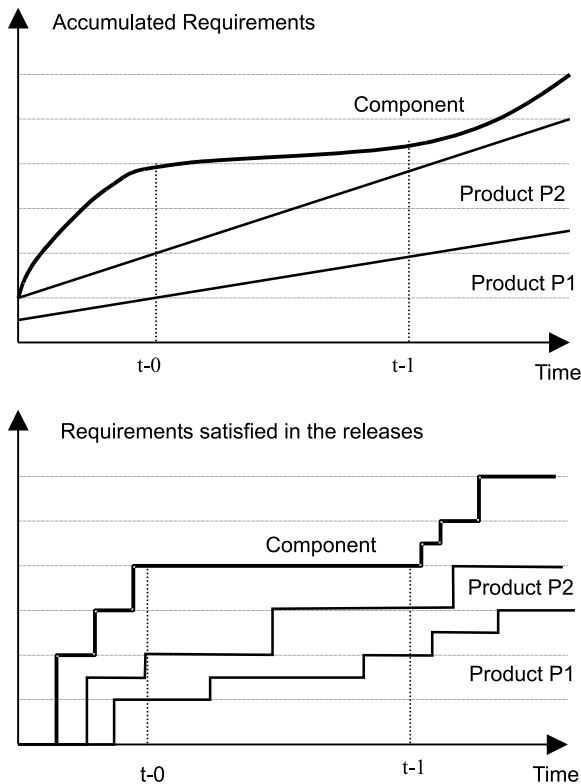
Fig. 3. To satisfy the requirements the reusable component must be modified more often in the beginning of their life.
