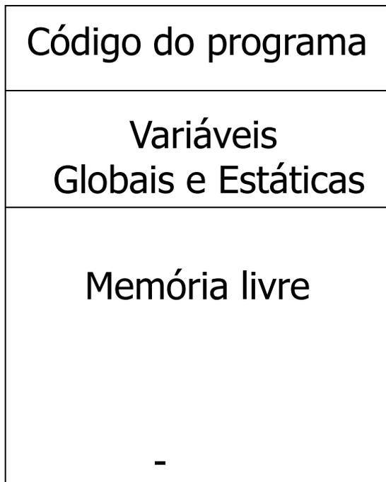
2) `v=(int*)malloc(10*sizeof (int));`
