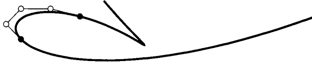
Figure 5.3 Convex hull property: a quartic Bézier curve is plotted for parameter values t \in [-1, 2] .
