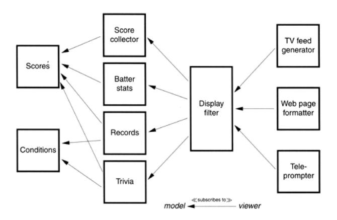
This kind of model-viewer network is a common (and valuable) design technique. Each link decouples raw data from the events that created it—each new viewer is an abstraction. And because the relationships are a network (not just a linear chain), we have a lot of flexibility. Each model may have *many* viewers, and one viewer may work with multiple models.
