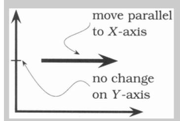
In computing, the term has come to signify a kind of independence or decoupling. Two or more things are orthogonal if changes in one do not affect any of the others. In a well-designed system, the database code will be orthogonal to the user interface: you can change the interface without affecting the database, and swap databases without changing the interface.
