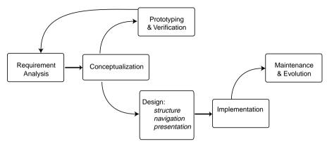
Figure 1. The lifecycle of a Web application.
