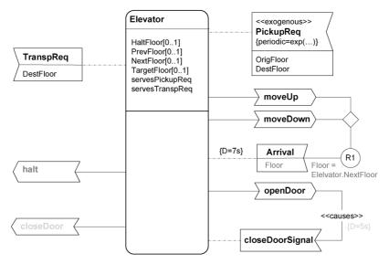
Fig. 4. A simulation model for the elevator system.
