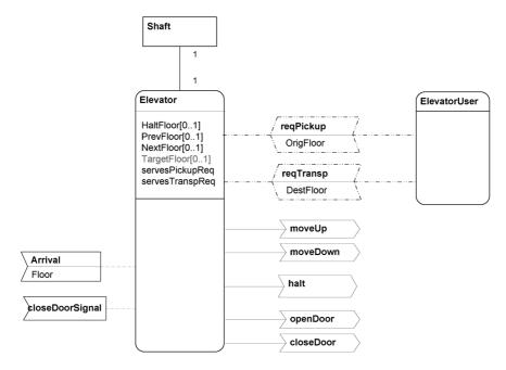
Fig. 3. An elevator scenario as an external AOR model.
