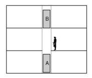
Fig. 5. Two elevators operating in one shaft.
